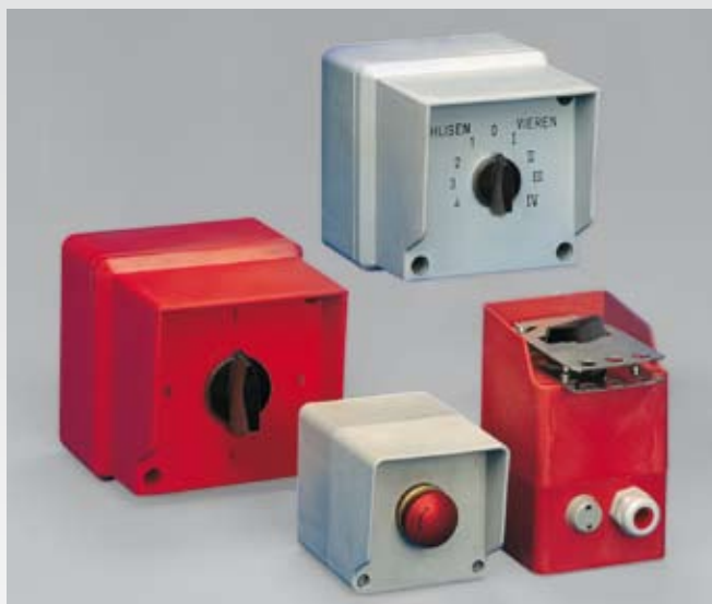
Top right: Citadel '7K' case with directly engraved position indications. Bottom left: Direct current emergency switch in special colour. Bottom centre: Push button in '1K' enclosure. Bottom right: Switch in '1K' enclosure with air relief valve.
